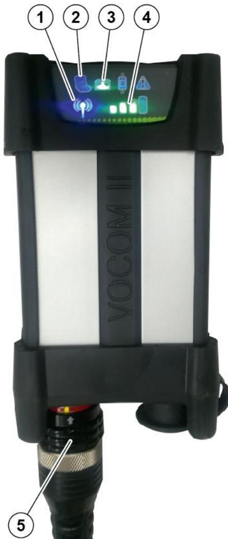
Fig. 4-4: VOCOM II function indicators in WLAN operation mode
