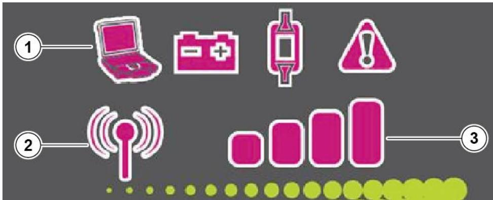
Fig. 4-3: VOCOM II front label with link status indicators
