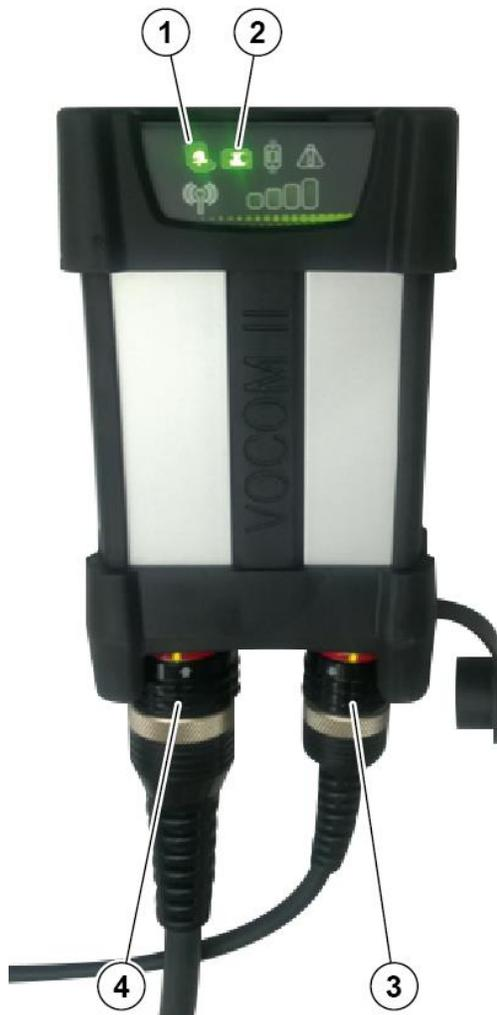
Fig. 5-1: VOCOM II function indicators in USB operation mode
