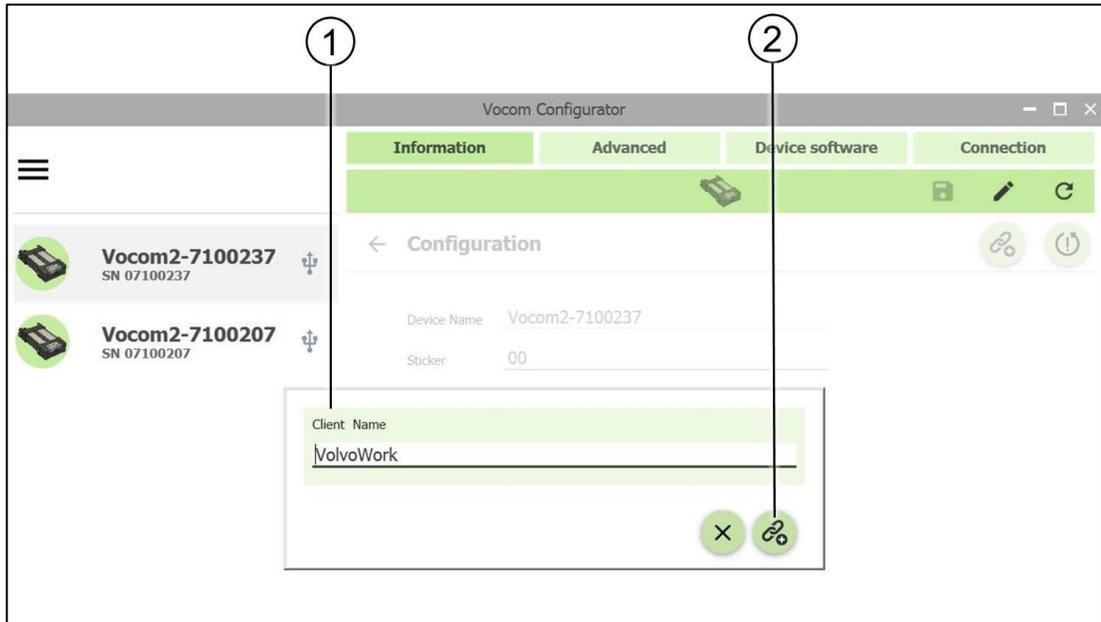
Fig. 6-7: Pairing a VOCOM II device with a client PC
